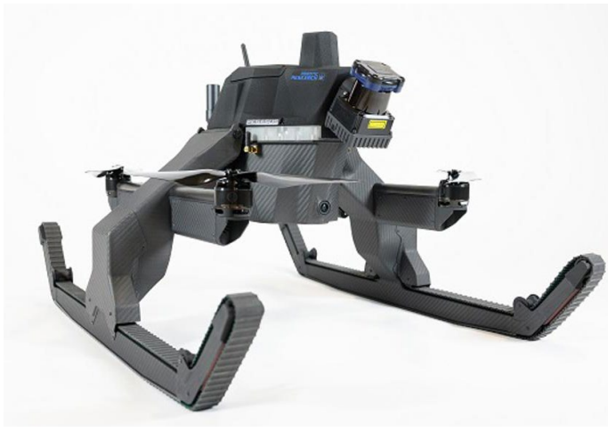
Robotic Research Pegasus IIe drone with skids deployed down to serve as treads.
